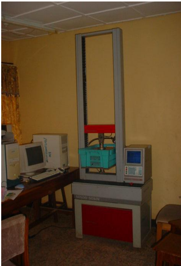
Fig. 1. Compression of tomatoes in plastic crate using Testometric Universal Testing Machine. (UTM).
